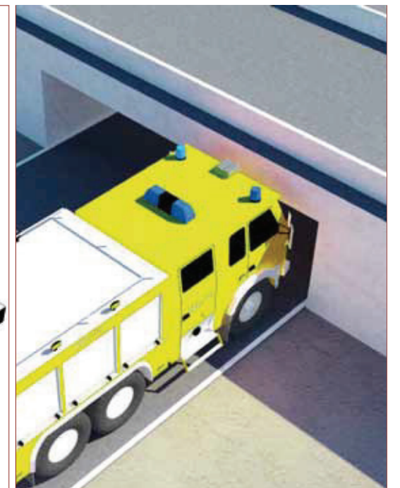
Inadequate clearance heights under bridge structures
